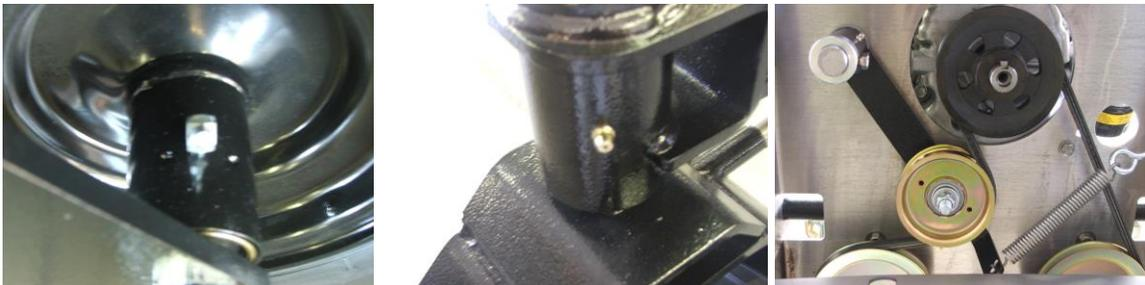
Inspect wheel and caster assembly every 25 hours for bearing wear, damage, debris, and proper installation.
